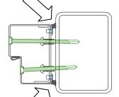
11. Apply mastic or flashings to seal frame to building. Fire rated doorsets must be sealed as shown, all round the frame, using either:
