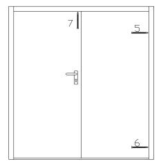
7. Close the active leaf again, then fit the last 2 fixings into face 5 of the fixed leaf jamb and 1 fixing into the head.
