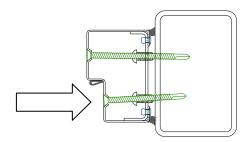
8. Open the doors fully, then tighten the 2nd set of frame adjusters in the reveals.
