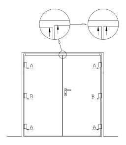
2. Align and grip the doorset in the opening, using the frame adjusting screws A in the corners, then the middle adjusters B.
