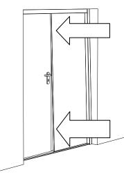
5. Using long countersunk frame fixings, first fix as shown, with 3 fixings in the active leaf jamb and 1 in the fixed leaf jamb.
