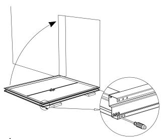
**1.** Assemble the doorset in front of the opening.
